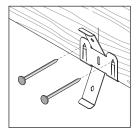
1 Attach bracket to joist using hammer tabs & nails
