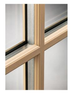
The Traditional SDL bars are injection molded along with our Evolve® Frame to eliminate separate application of the SDL bars. This all-in-one design offers a better flush-to-glass fit.
