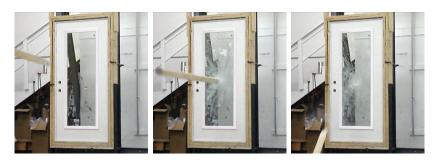
The Level D missile impact test fires an 8-foot long 2"x 4" at 50 feet-per-second at the door glass and door slab. The entire unit must remain intact through 9,000 pressure cycles, and also pass water-infiltration, structural loading, and forced air-infiltration tests.
