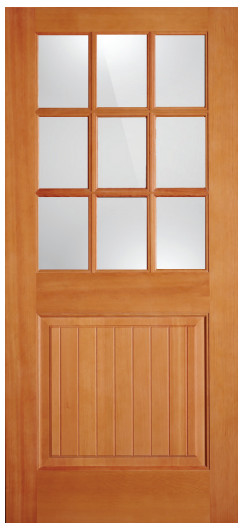
F37224 Low-E 7/8" SDL Bar 1-7/16" Beaded V-Groove Double Hip Raised Panel Wide Layout Ovolo Sticking 2/8 x 6/8 3/0 x 6/8 2/8 x 7/0 3/0 x 7/0
