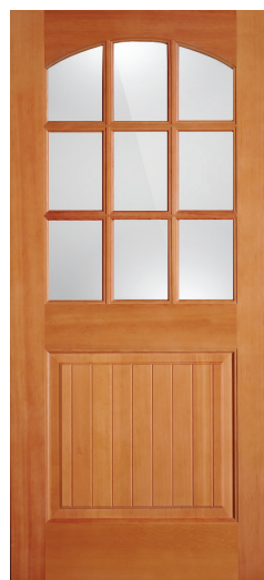
F37214 Low-E 7/8" SDL Bar 1-7/16" Beaded V-Groove Double Hip Raised Panel Wide Layout Ovolo Sticking 3/0 x 6/8
